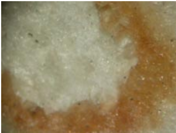
Figure 4 Gelatinized (yellow glasslike) fibres on the edge of a wormhole.
